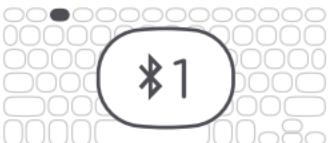
To pair a second device, press and hold the Bluetooth 2 button for three seconds, and follow the same procedure.
