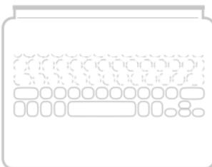
The folio-style flap (attached to the case) is also magnetized. It has a light magnetic attachment to the back of the keyboard. It allows the keyboard to slide along the flap to form a stand but prevents the keyboard from slipping.
