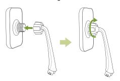
Insert the tabs at the bottom of the arm into the openings on the base so that the arm snaps into place. NOTE: This connection is permanent. Once you assemble the base you cannot disassemble it.
