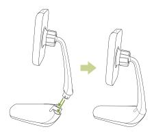
4. Pass the included cable's micro-USB jack through the rear of the opening on the desk mount base and connect it to the port on the bottom of the desk mount charging pad. Connect the cable's larger USB jack to a wall-charging adapter with at least a 1.8-amp output.
