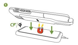
Make sure that the charge force adapter is centered on the charging base. (When charging from a mophie charge force mount the charge force adapter will automatically align itself for a proper charge.) Charging will begin automatically.
