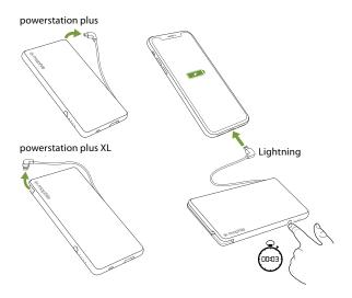
Your powerstation plus/powerstation plus XL portable battery also has a USB-A port that is compatible with most USB devices and wearables. Connect the USB cable included with your device to the powerstation plus/powerstation plus XL portable battery's USB-A port and to your device. Press the status button for 3 seconds to begin charging. You can connect devices to the portable battery's USB-A port and to its integrated Lightning cable at the same time.
