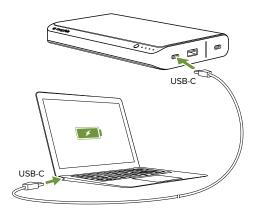
IMPORTANT: Do not connect a USB-C equipped laptop to the powerstation USB-C 3XL battery's USB-A port.
