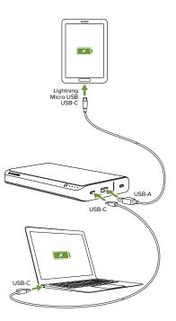
When charging multiple devices, the powerstation USB-C 3XL battery's USB-C output port will deliver power levels up to 30W to a compatible device, and its USB-A output port will deliver power levels up to 12W to a compatible device.
