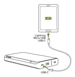
The powerstation USB-C 3XL battery's USB-A output port will deliver power levels up to 12W when connected to a compatible device.
