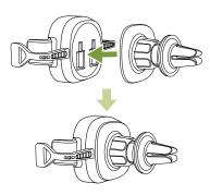
Connect the supplied micro-USB cable to the vent mount's micro-USB port and to the supplied QC 2.0 car charger's USB-A port. Insert the car charger into your vehicle's 12-volt power outlet.
