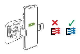
IMPORTANT: DO NOT DIRECT HEATED AIR FROM THE VENT ONTO THE VENT MOUNT WHILE IT IS ATTACHED TO THE VENT—this can damage the vent mount and an inserted device. When running the vehicle's heater, completely close the vent the vent mount is attached to, or direct the heated air out of the vehicle's lower vents and entirely away from the upper vents.
