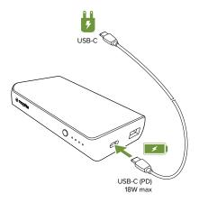
The USB-C port will charge the powerstation PD XL or powerstation PD battery at USB-C PD fast-charging speeds when connected to a compatible wall charger.
