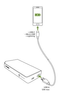
When charging devices from the USB-C and USB-A ports at the same time, the powerstation PD XL and powerstation PD batteries can deliver up to 18W via their USB-C port and up to 5W via their USB-A port.
