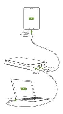
When charging multiple devices, the powerstation pro XL battery's USB-C output port will deliver power levels up to 30W to a compatible device, and its USB-A output port will deliver power levels up to 12W to a compatible device.
