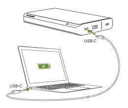
IMPORTANT: Do not connect a USB-C equipped laptop to the **powerstation pro XL** battery's USB-A port.
