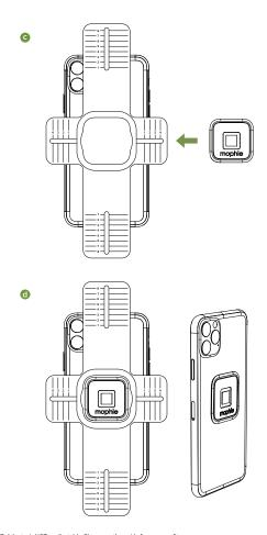
NOTE: Adapter is NOT readjustable. Please use the guide for a proper fit.
