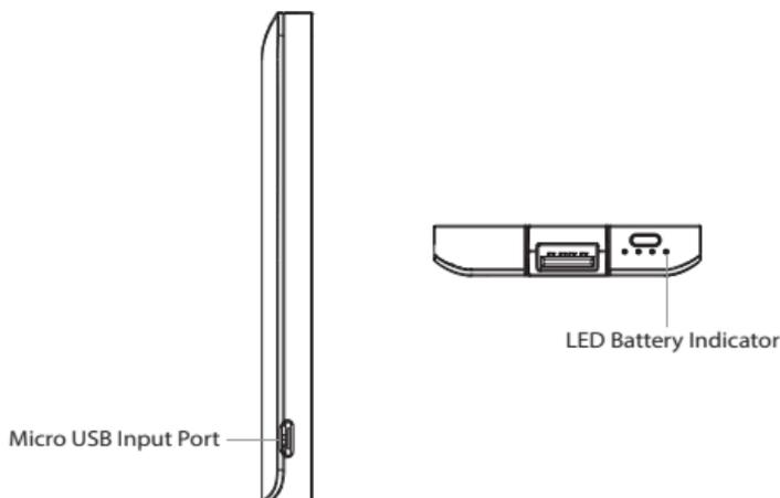
While charging, the LED battery indicator will illuminate. When battery is fully charged, the power indicator will display four solid blue lights. When fully charged, disconnect the USB to Micro USB Cable.
