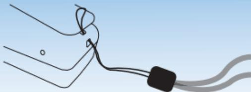
Step 1. Loop the thin end of the neck strap through the slot in the Headset.
