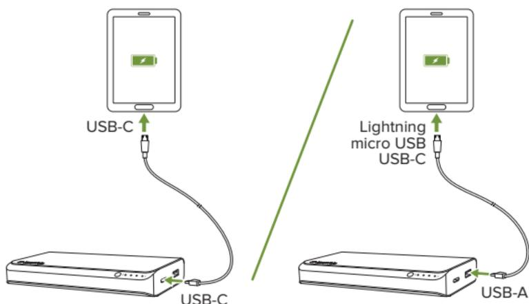
**IMPORTANT:** Do not connect a USB-C equipped laptop to the **powerstation pro** battery's USB-A port.
