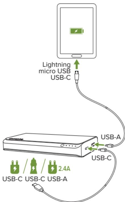
**IMPORTANT:** Do not connect a USB-C equipped laptop to the **powerstation** battery's USB-A port.
