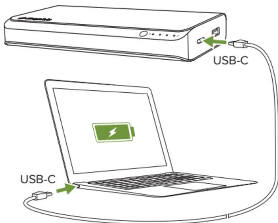
**IMPORTANT:** Do not connect a USB-C equipped laptop to the **powerstation pro** battery's USB-A port.
