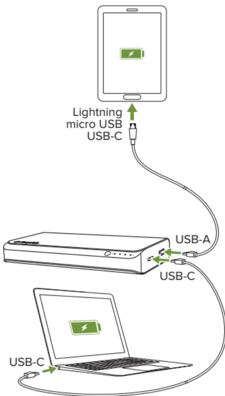
**IMPORTANT:** Only connect a USB-C equipped laptop to the **powerstation pro** battery's USB-C port. Do not connect it to the USB-A port.
