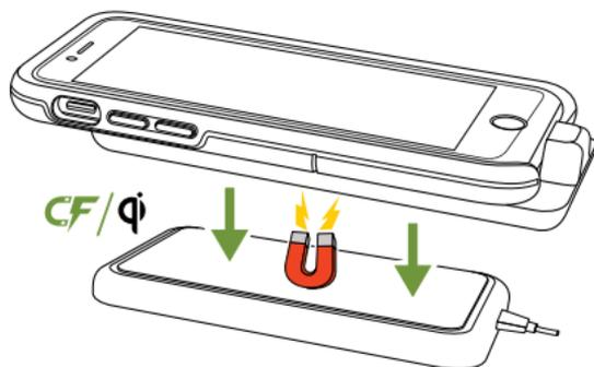
2. Make sure that the **charge force battery** is centered on the charging base. (When charging from a mophie charge force mount the **charge force battery** will automatically align itself for a proper charge.)
