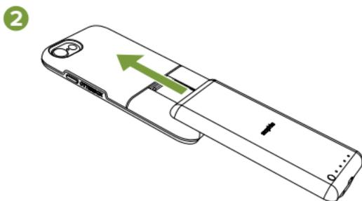
3. Slide the battery all the way up onto the case until the lock button clicks into place.
